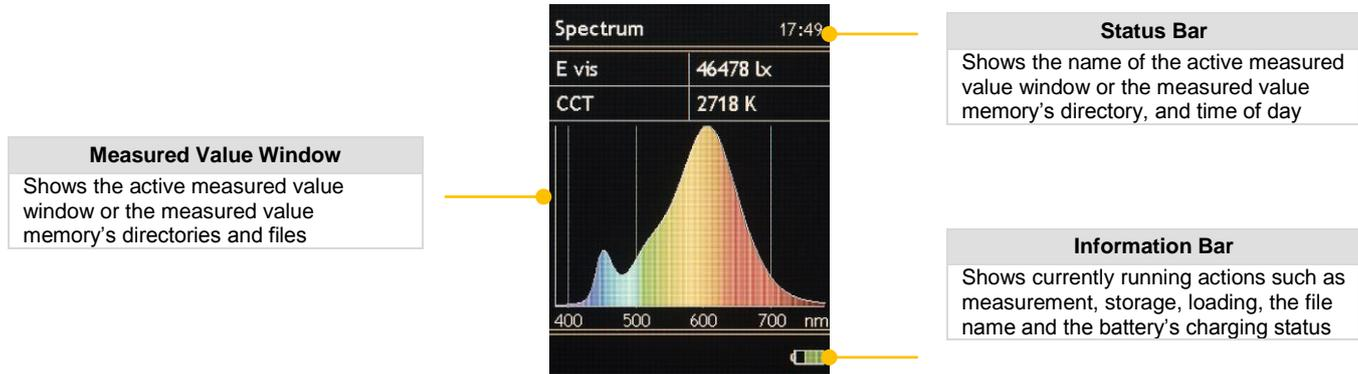
The battery icon in the information bar shows the charging status of the battery, or indicates operation with mains power or power from the PC. Even when the device is switched off, the charging status LED indicates whether the battery is being charged or has already been fully charged.
